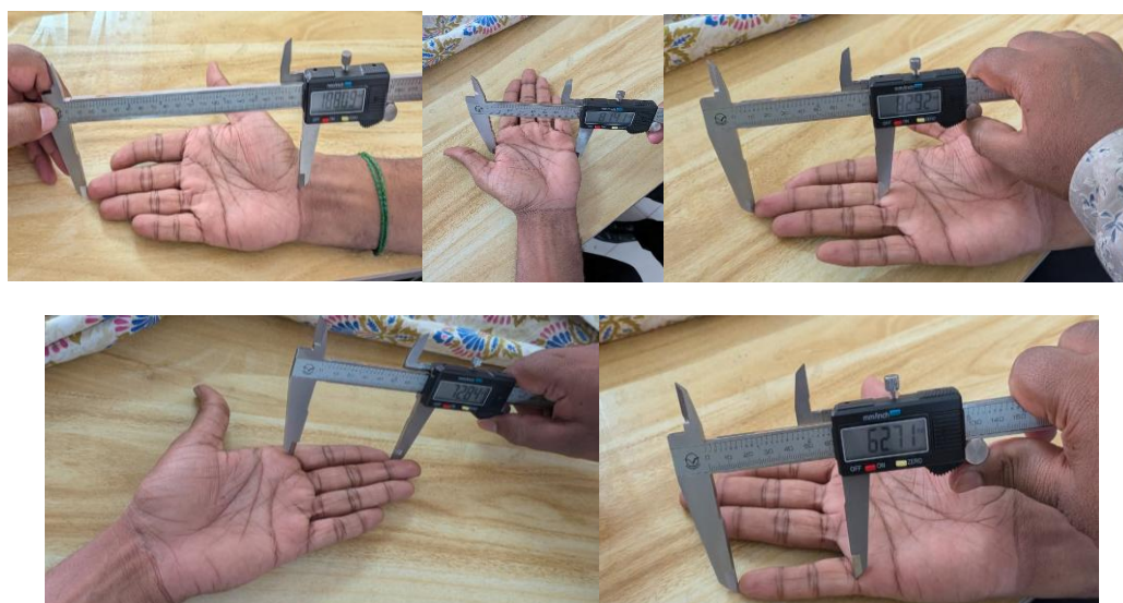
Figure 1. Measurement of hand and finger dimensions using a digital Vernier caliper.
